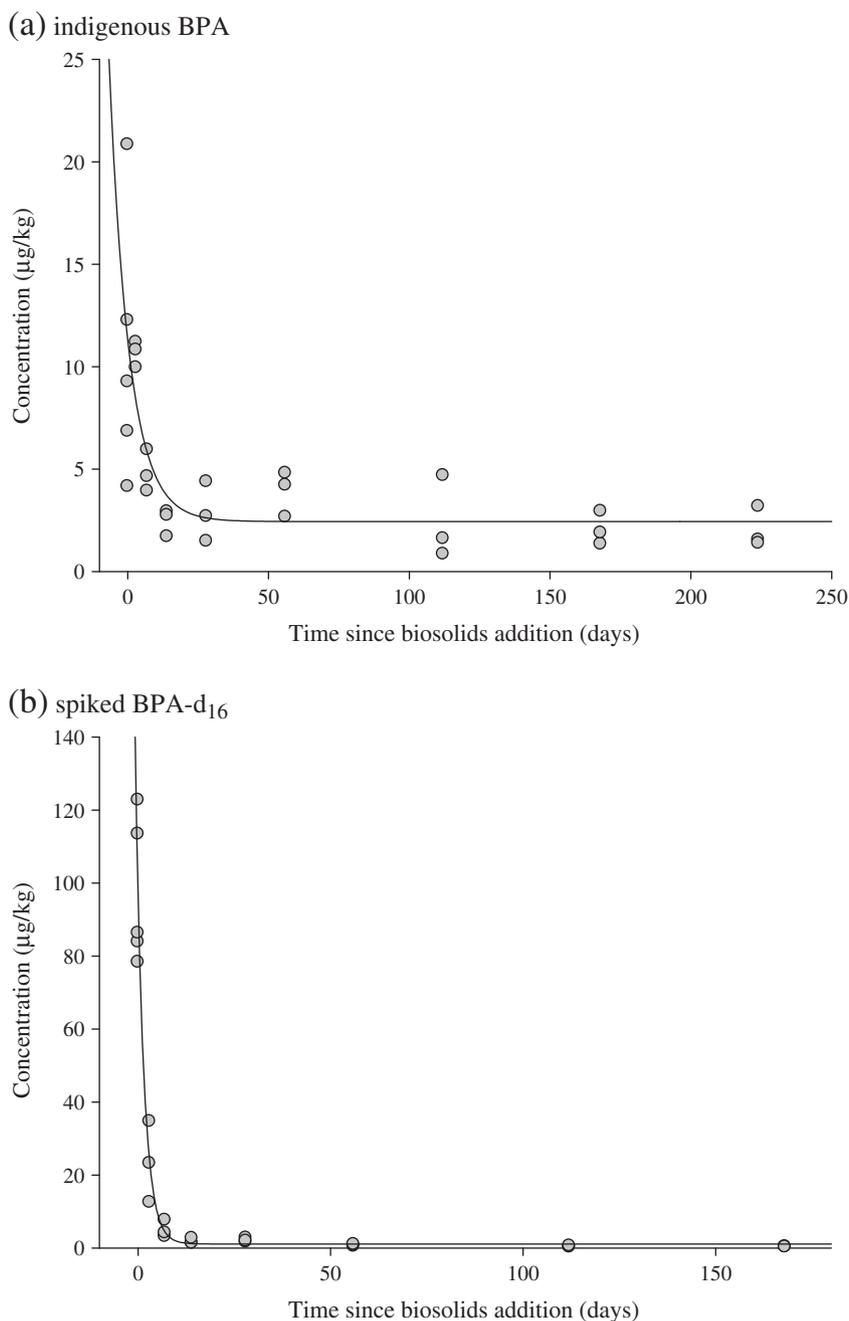
**Fig. 2.** Degradation of (a) indigenous BPA and (b) spiked BPA-d<sub>16</sub> following the addition of lagoon dried biosolids (LDB) to a soil, with the fit of a biphasic degradation model. Note that (b) only presents data for the duration of the experiment where the compound was above the limit of detection.
