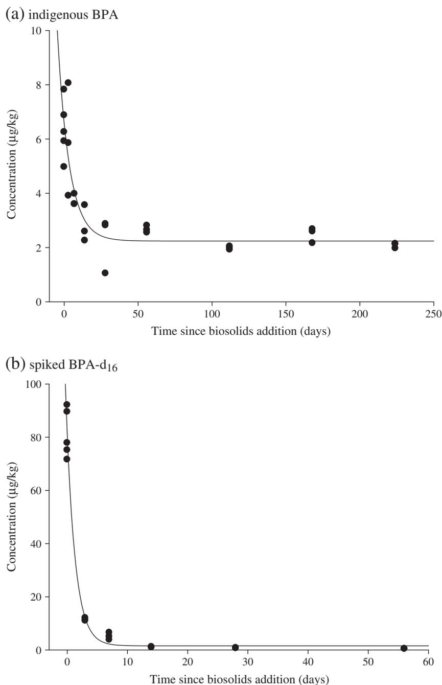
**Fig. 1.** Degradation of (a) indigenous BPA and (b) spiked BPA-d<sub>16</sub> following the addition of centrifuge dried biosolids (CDB) to a soil, with the fit of a biphasic degradation model. Note that (b) only presents data for the duration of the experiment where the compound was above the limit of detection.
