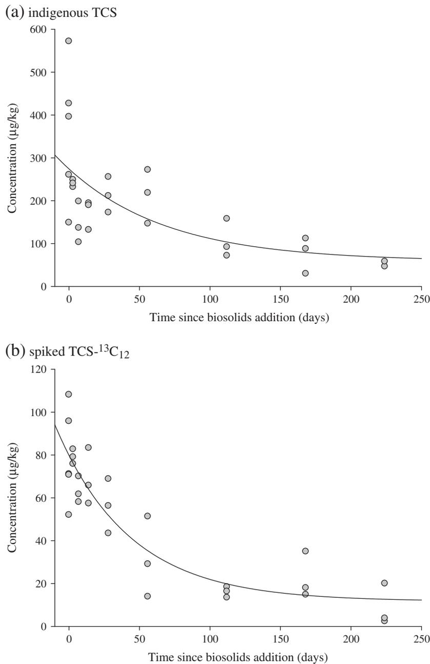
**Fig. 4.** Degradation of (a) indigenous TCS and (b) spiked TCS-<sup>13</sup>C<sub>12</sub> following the addition of lagoon dried biosolids (CDB) to a soil, with the fit of a biphasic degradation model.
