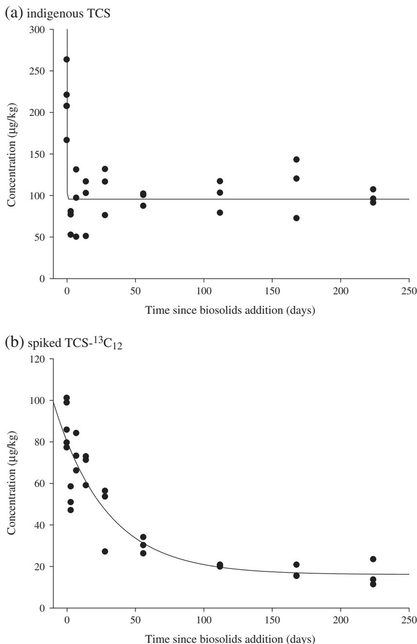
**Fig. 3.** Degradation of (a) indigenous TCS and (b) spiked TCS-<sup>13</sup>C<sub>12</sub> following the addition of centrifuge dried biosolids (CDB) to a soil, with the fit of a biphasic degradation model.
